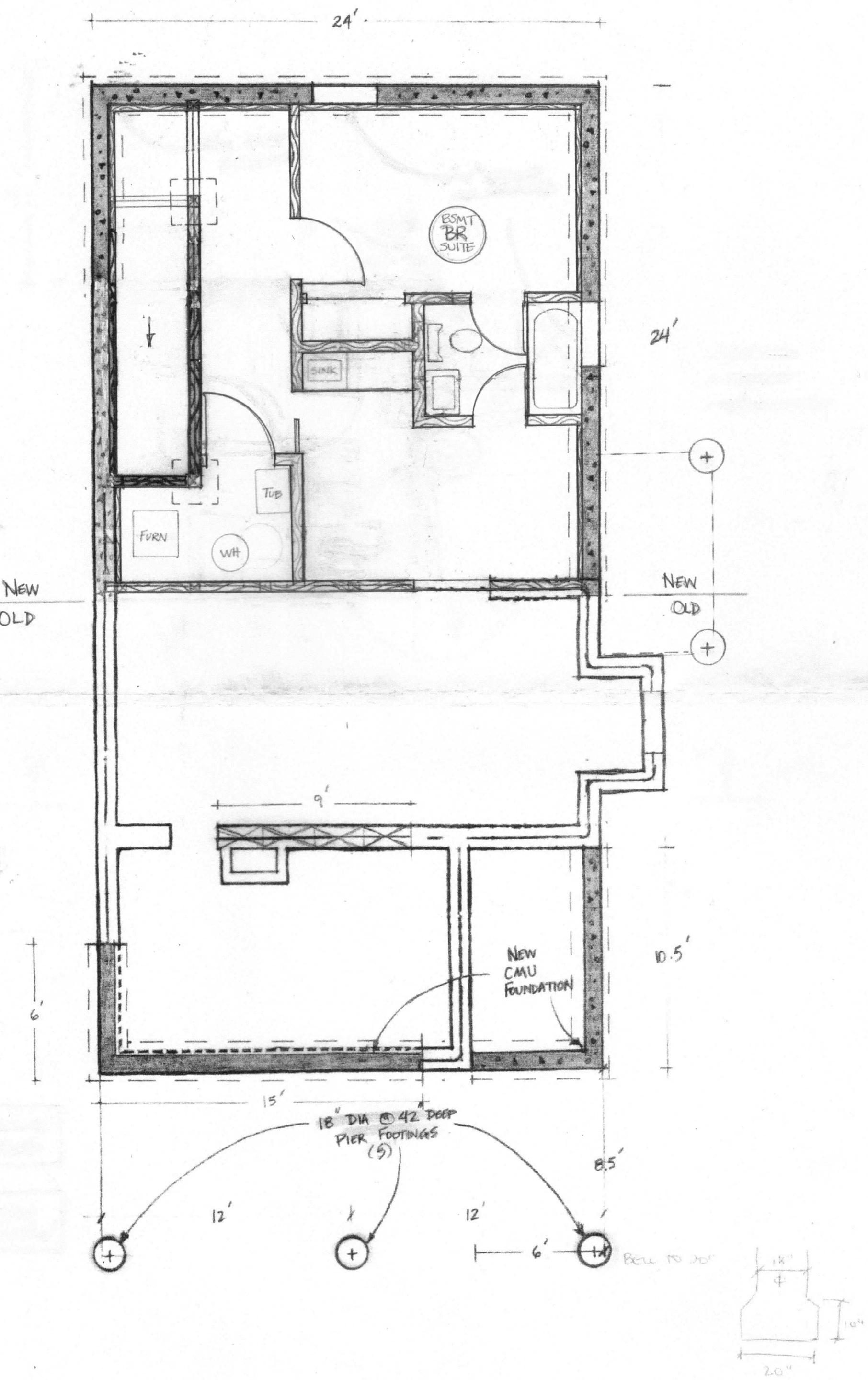
Walls closer than five feet from adjacent property line shall have minimum 1 hour fire-resistance rating with exposure from both sides. R302.1
